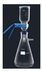
Filtration equipment is ideal for separating the drying agent from an organic solution. Furthermore, the systems can be used safely under a vacuum with the aid of a water jet pump with check valve. It should be noted that these kits are fully autoclavable, so they are an ideal choice for HPLC solvent preparation and microbiology applications.
